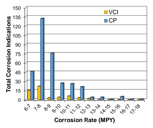
Figure 6. Total number of corrosion indications per corrosion rate segments of all (12) tank floors.
